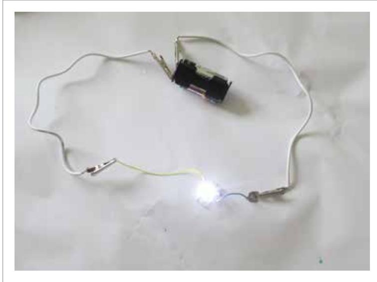
**Figure 13. Complete circuit**
