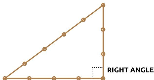
**Figure 16. Surveyor's rope laid out to form a right-angled triangle**
