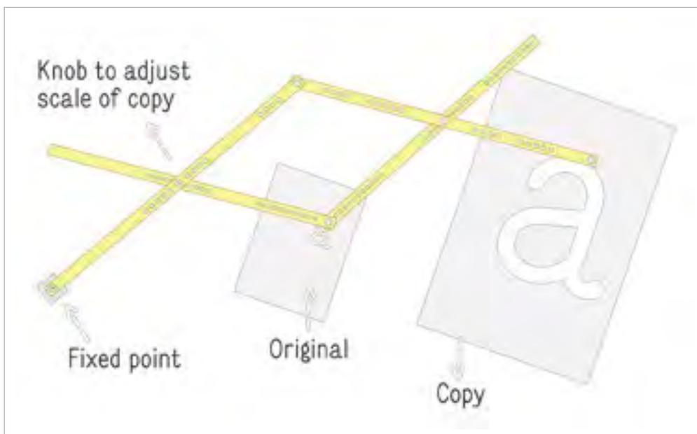
Figure 48. Pantograph. A mechanical tool that can be used for scaling images.
