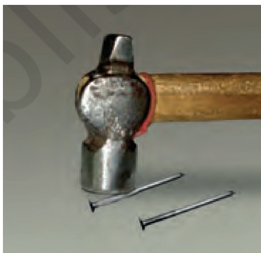
Fig. 2.4: Testing malleability of metal
